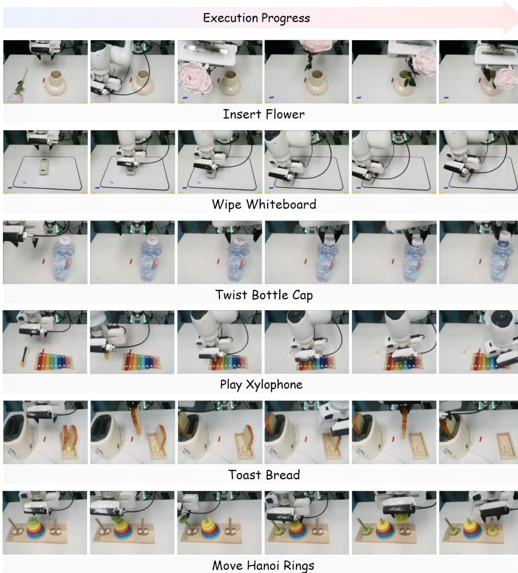
Figure 9: Robot execution progress in real-world tasks. We visualize key frames of the robot’s execution process from the front camera view in real-world tasks.
