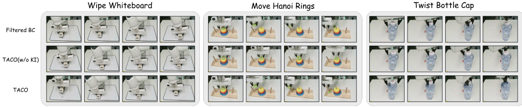
Figure 11: Failure case analysis. Representative rollouts of Filtered BC, TACO (w/o KI), and TACO on Wipe Whiteboard , Move Hanoi Rings , and Twist Bottle Cap . The two baselines fail at contact transitions in complementary ways, whereas TACO completes all three tasks.
